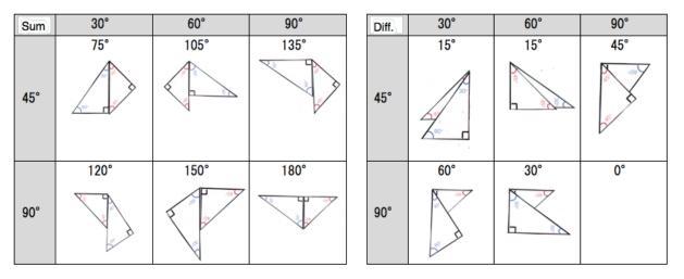
The table above does not show how a 90° angle can be made. However, one can be made outside of set square pieces as shown below (Fig. 1). In addition, a 165° angle can be made if we use 3 pieces of set squares (Fig. 2). A 165° angle cannot be made by using only a pair of set squares, however, if you can draw an auxiliary line, it is possible to create a 165° angle.
